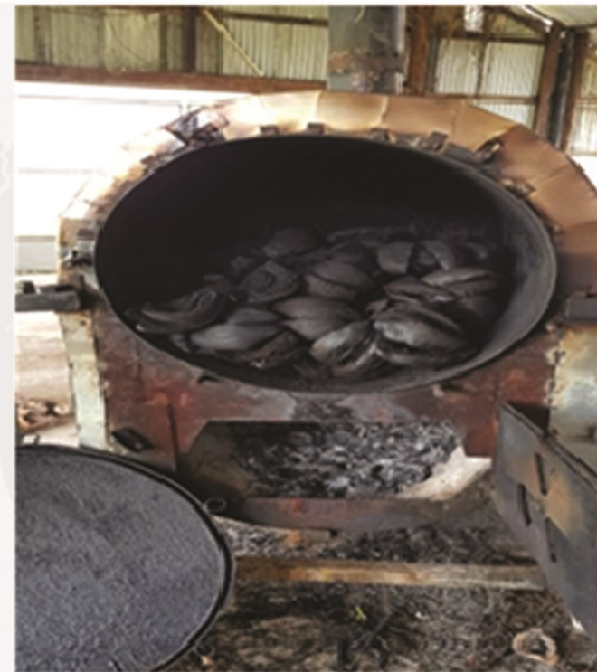
Production of cocnut husk biochar using the kilt
